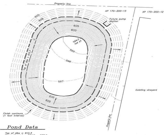
Top of dike = 610.3 Floor of pond = 594.0 - 598.0 High water = 608.5 Maximum depth = 14.5 feet Storage to 608.5 = 7.8 ac ft Surface area at 608.5 = 0.88 acres
